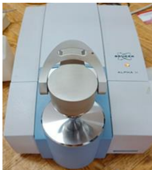
Figure 2: Shape ATR-FTIR device used
