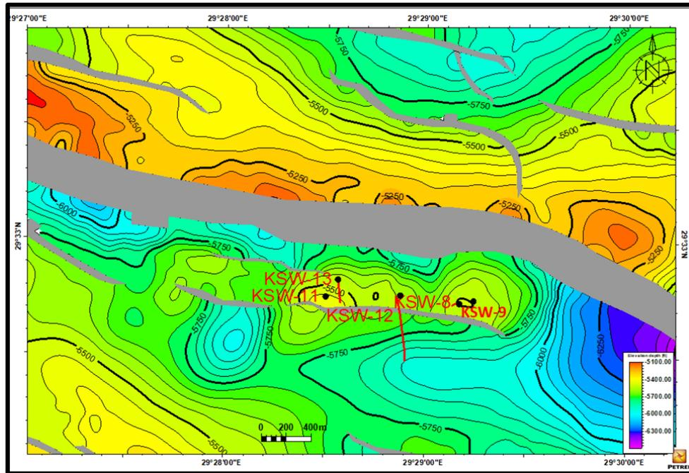
Figure 16: Depth Structure Contour map on top Abu Roash "C" Member.
