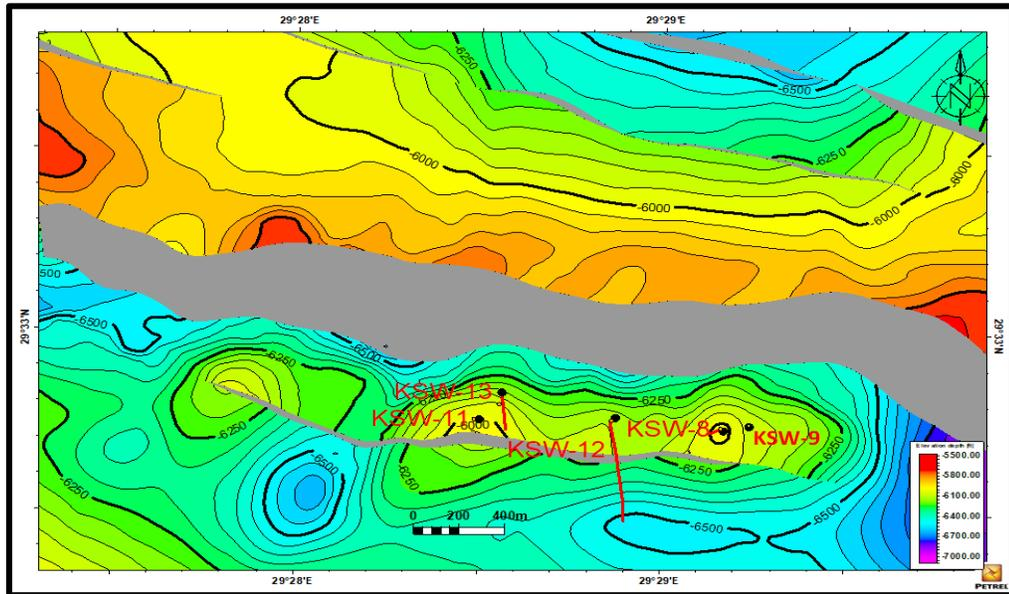
Figure 14: Depth Structure Contour map on top Abu Roash "G" Member.
