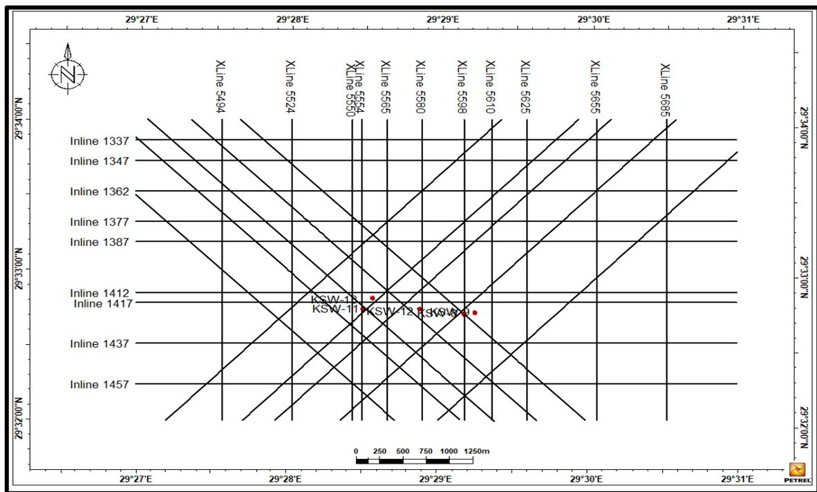
Figure 10: Base map of 3D seismic line among Karama SW field.
