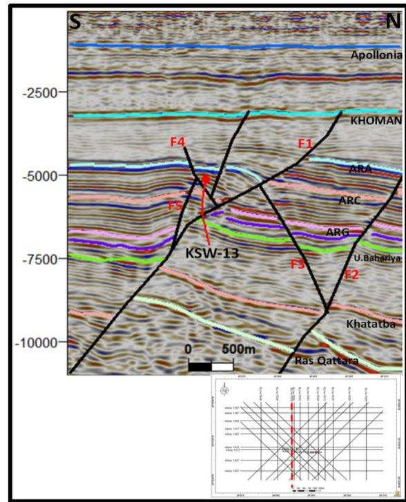
Figure 12: N-S Seismic Cross Line 5550
