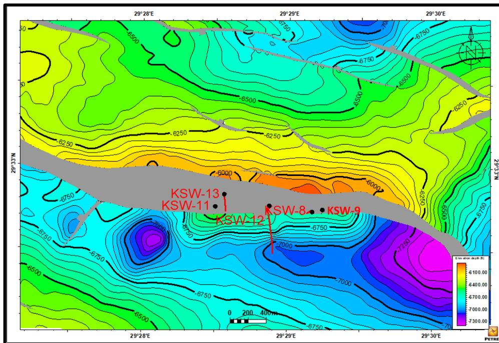
Figure 15: Depth Structure Contour map on top Abu Roash "E" Member.
