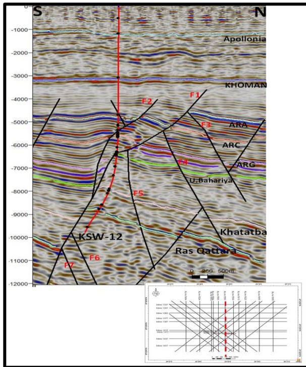
Figure 11: N-S Seismic Cross Line 5581
