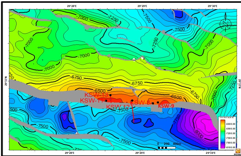
Figure 13: Depth Structure Contour map on top Upper Bahariya Formation.
